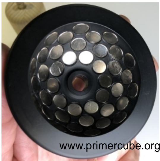
All 40 magnets in place.
