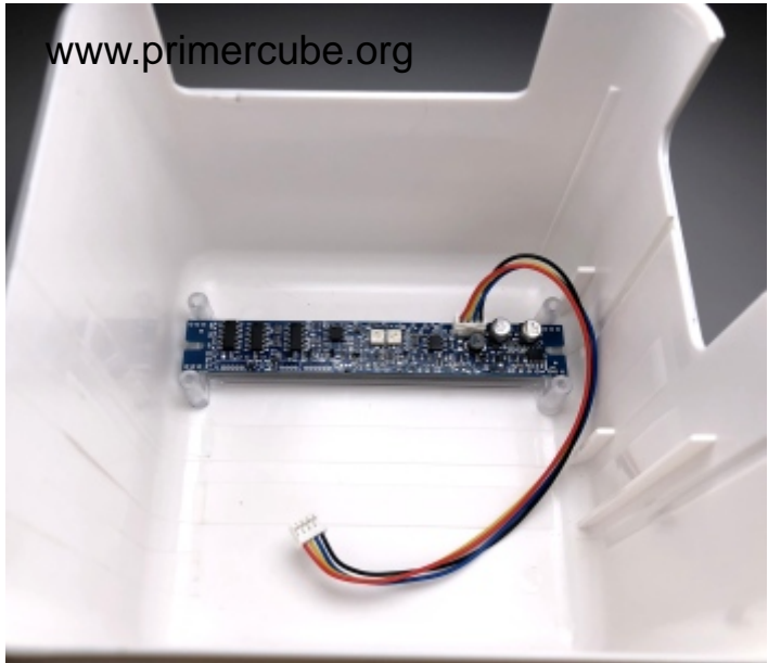
The Barmeter display that was previously calibrated is placed into PC 7100 as shown in the image to the left.
